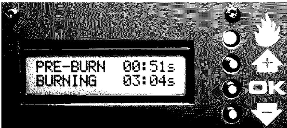
The display gives the user information about the status and adjustment of the burner. The burner has two menus and in order switch from one to another you have to press the “+” and “-“buttons simultaneously.
